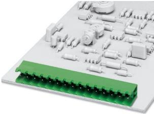
Header, nominal current: 12 A, rated voltage: 250 V, pitch: 5.0 mm, no. of positions: 12, mounting: Soldering
